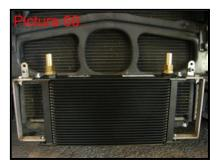
• Now you will see 4 free bolts sitting on the frame in front of the radiator. The front heat exchanger element is installed on the two lower bolts (*Pic.67*). The front element comes preassembled, but you might have to loosen the bolts a little to make it fit. The two L shaped brackets are installed onto the free bolts (*Pic.68 and Pic.69*). Secure them with supplied ESS nuts and washers using a 13mm socket. Tighten all the bolts on the element assembly.
