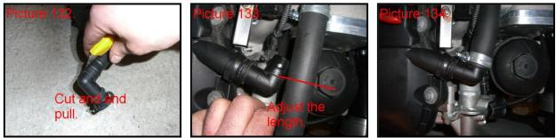
Step 16: Install rear engine cover, brake booster hose, cover around brake booster and fuel valve.
